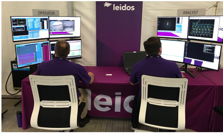
Shown is the optional shore station for Leidos' autonomous hydrographic survey system. The left operator supervises the vessel and payload. The right analyst receives live bathymetry from the vessel and initiates processing and quality assurance. (Photo courtesy of Leidos)
